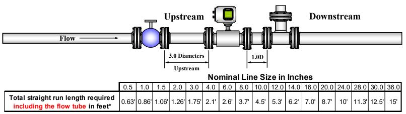
\* Straight run length includes: 4.0 pipe diameters (3.0 up and 1.0 down) from the flow tube flanges plus the length of the flow tube.
