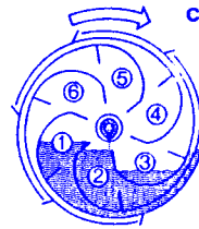
Compartment No.1 ready to empty. Compartment No.2 full and overflowing into Compartment No.3.
